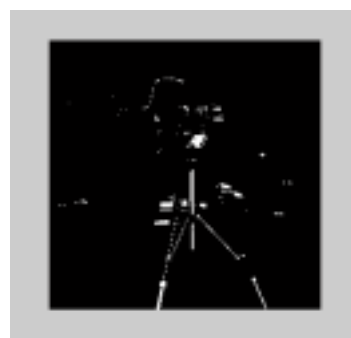
Fig.8 Thresholding image using maximum entropy principle. ( th = 193 )
