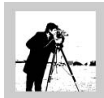
Fig.7 Thresholding image using Otsu's method. ( th = 89 )
