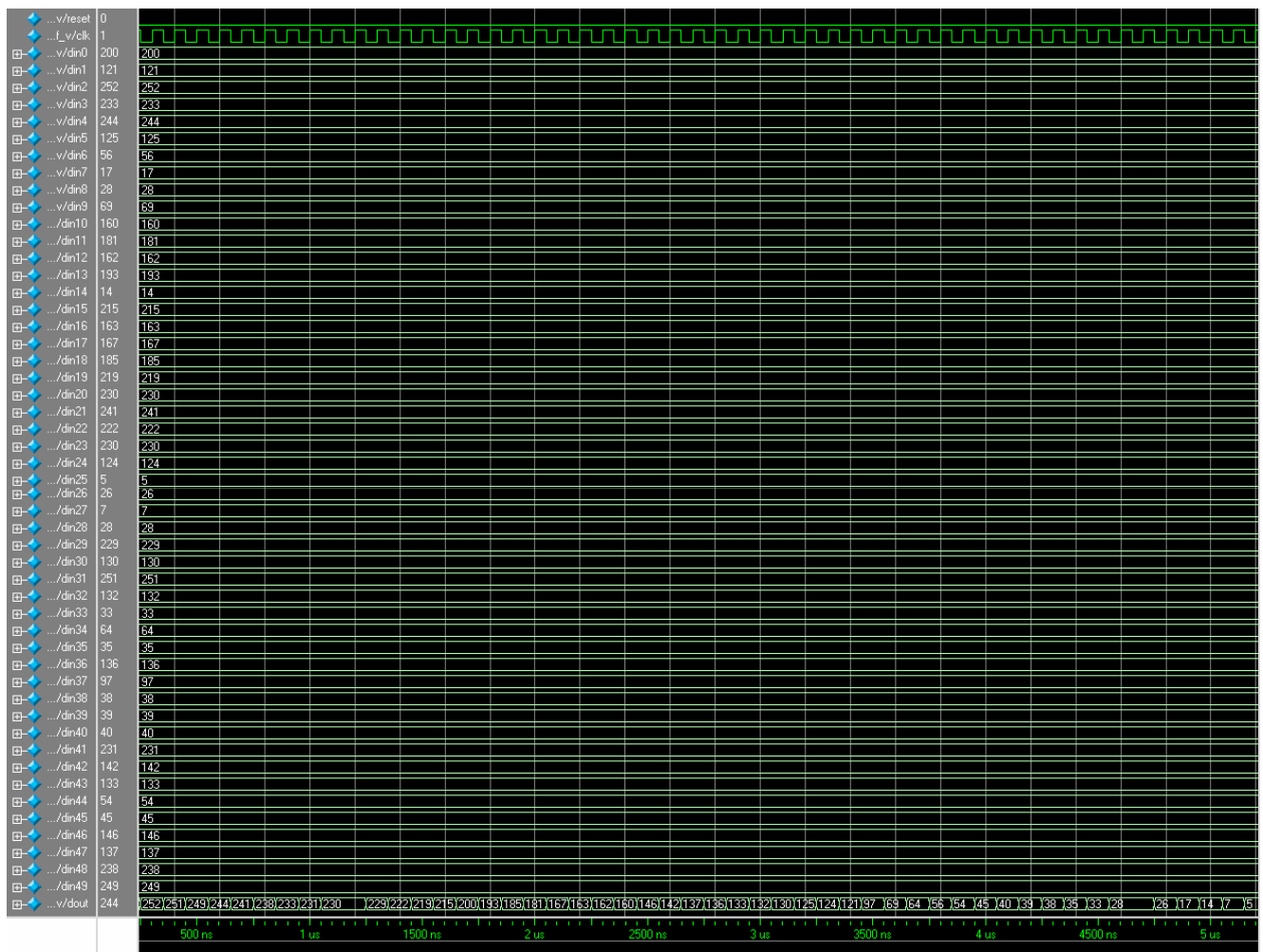
Fig.2. VHDL Simulation of the proposed 50 number sorting algorithm
