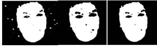
(a) (b) (c) (a) After the binary image (b) Corrosion (c) Expansion Fig.3. The result of erosion and dilation
