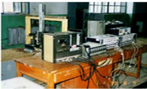
Figure 4 Hardware composing of the traditional measuring system for bionic plough
