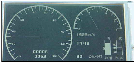
Figure 5. the Interface of the new vehicle digital instrument interface
